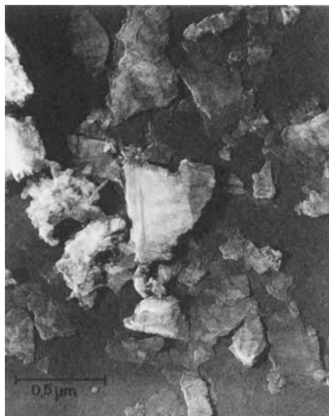
Fig. 5. Electron micrograph of 'active' dimer hydroxide suspended in \text{H}_2\text{O} , after ultrasound treatment and drying on carbon grid. Cr-shadowed, 40°; magnification 50000 \times .
